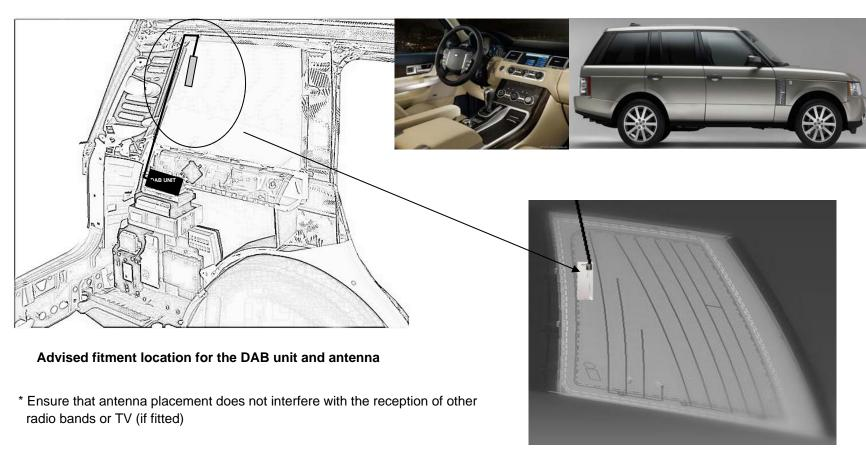
\*\* If the windscreen is selected for antenna placement then ensure that it does not have a heating element. With a fitted heating element then the antenna must be fully contained within the element free area adjacent to the A-pillar – care must be applied for such placement.
