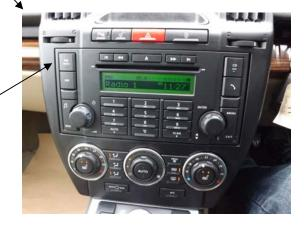
Head Unit **MUST** have this button identification for applicability to upgrade to DAB
